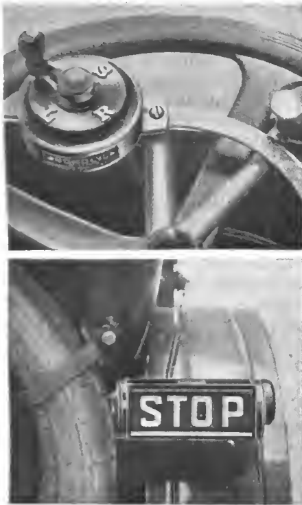
Above—Control of Nokolyd electric signal Below—Nokolyd signal mounted on car
